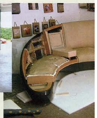
9. The upholstery is a traditional assembly of springs and wadding covered with stone-coloured leather hide
