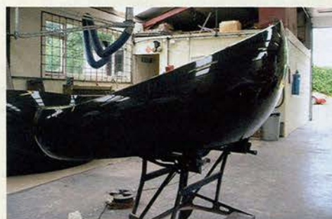
8. Completed sections polished using polyurethane lacquer and cut back to a full gloss using fine cutting paste and lambs' wool bonnets on hand-held polishers
